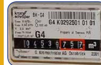
Write down all the numbers from left to right including any zeros. Ignore any numbers after the decimal point or which may be shown in red. Metric gas meters show gas used in **m<sup>3</sup> (cubic meters)** and have **five** numbers
