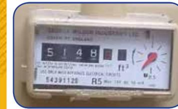
Write down all the numbers from left to right including any zeros. Ignore any numbers after the decimal point or which may be shown in red. Imperial gas meters are shown in **cubic feet** or **ft<sup>3</sup>** and have four numbers to
